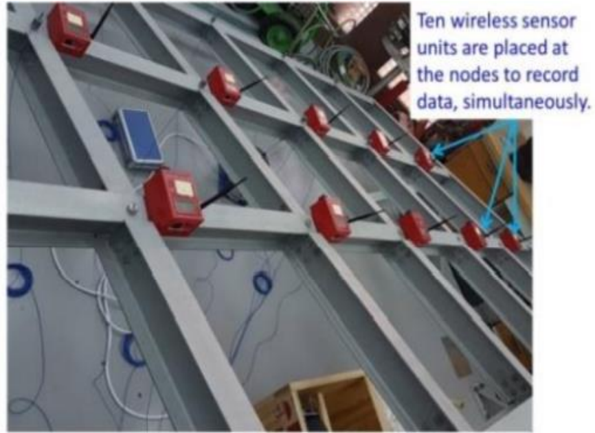
The test setup and wireless sensors used in Avci et al.
