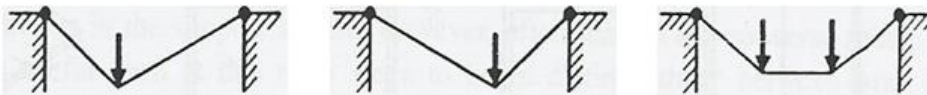
(b) Nonrigid or flexible structure (e.g., a cable). The shape of the structure changes with changes in the loading condition.
