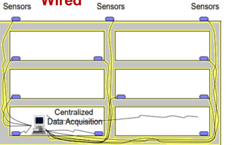
Traditional SHM system using centralized data acquisition.
