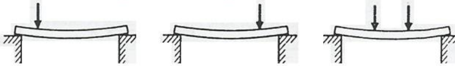
(a) Rigid structure (e.g., a beam). The structure is stiff and does not undergo appreciable changes in shape with changes in the loading condition.
