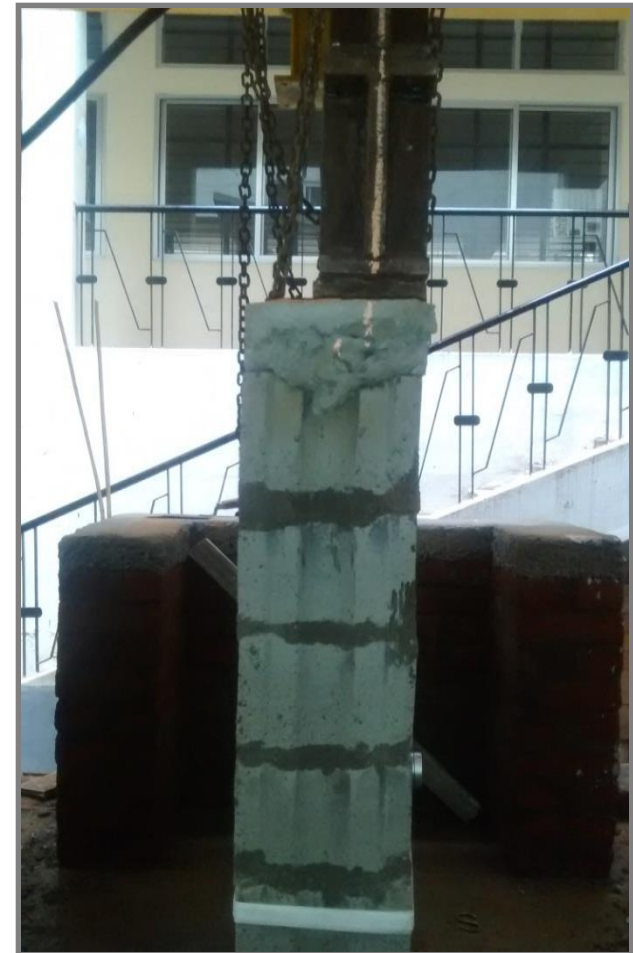
Fig: Ladder Arrangement for Axially & Eccentrically Loaded Geopolymer Hollow Block Wallete
