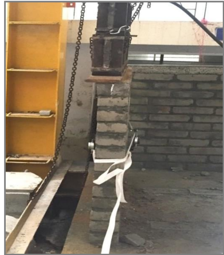
Fig: Ladder Arrangement for Eccentric Loading
