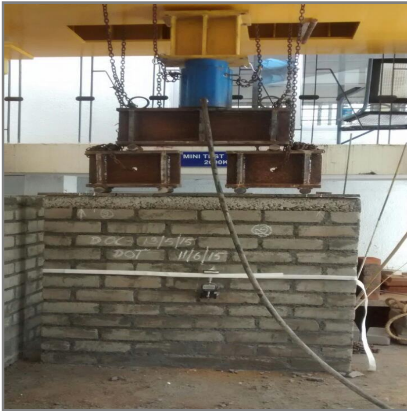
Fig: Ladder Arrangement for Geopolymer brick Wallete
