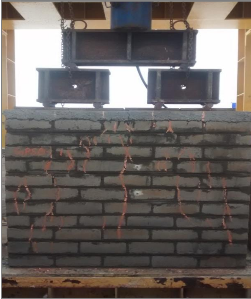
Failure Pattern of Axially Loaded Wallete
