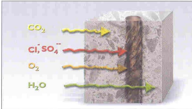
Corrosion of steel in OPC
