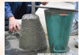
Fig. 2: Highly workable fresh concrete
