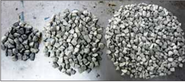
Fig 16 : Natural stone aggregate (extreme left) and 'nano concrete' aggregates (right) [41]
