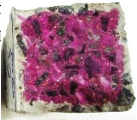
Fractured cross-section of a prism
