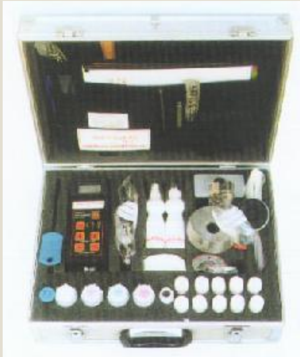
Chemical kit for field test on concrete Sudarshan S. Iyengar
