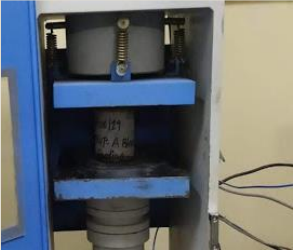
Close-up view of core specimen under test
