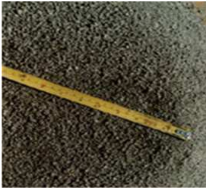
VSI Crushed Sand - Cubical - Good Quality
