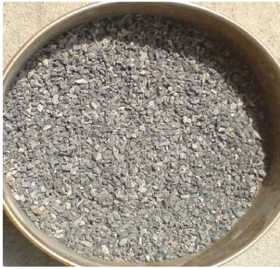
Poor Quality CS-Sand with Flaky Particles
