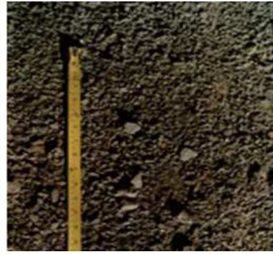
JAW Crushed Sand - Flaky - Poor Quality
