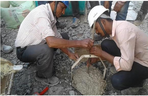
Img5 220mm slump without segregation
