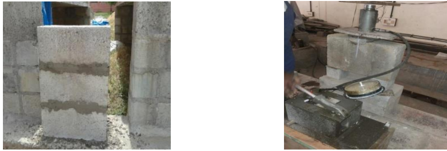
Fig. 10. Block masonry (400*190*150mm, 1:6 mortar mix)
