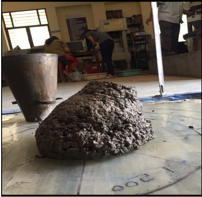
Slump in 100% pond ash replacement without SP
