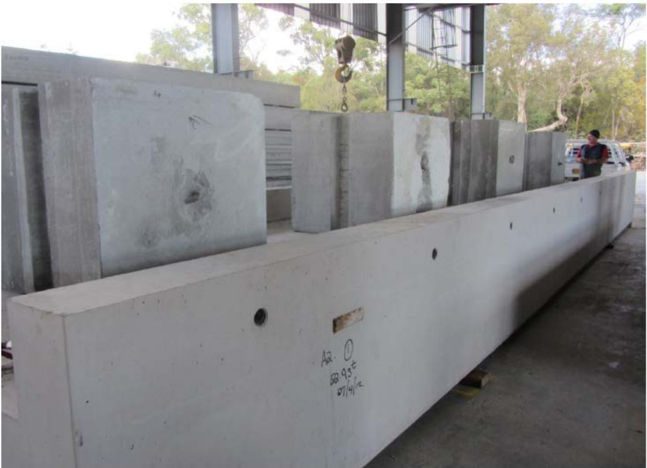
Load testing of a 10 metre precast geopolymer beam.
