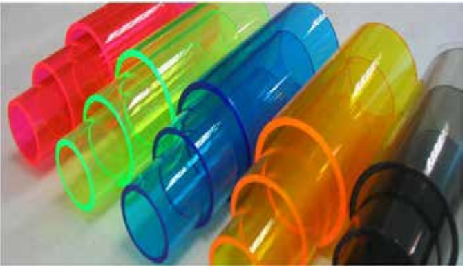
Polymethylmethacrylate / Acrylic (PMMA):Surfaces, Sinks
