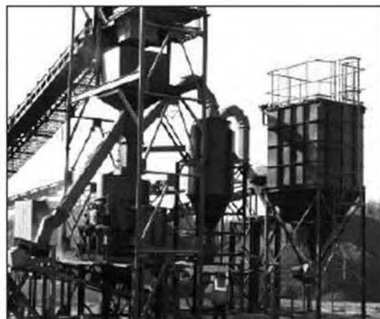
VSI with Air Filtering Technology (AFT)
