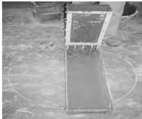
Photographs of fresh concrete tests on SCC
