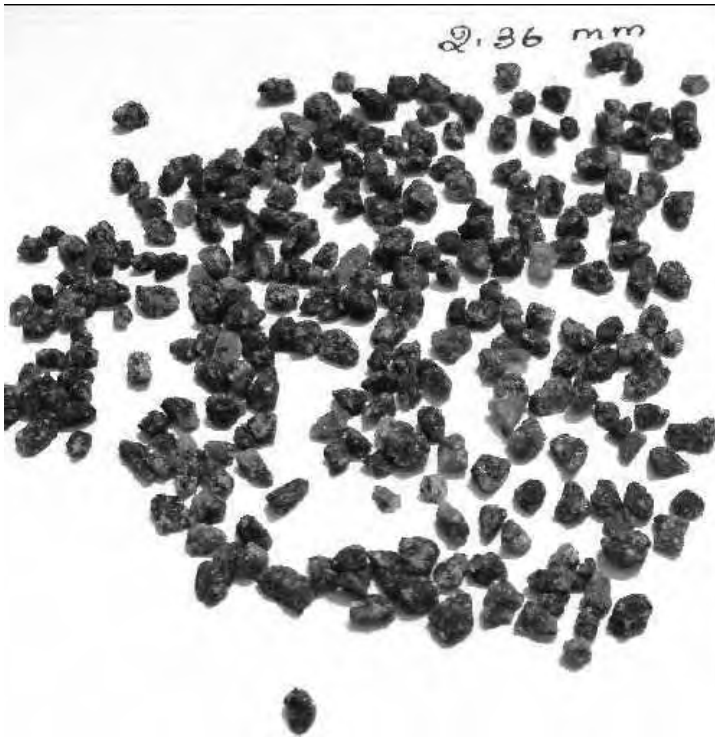
Shape of i-sand, the Manufactured sand equivalent to River Sand retained by 2.36mm sieve
