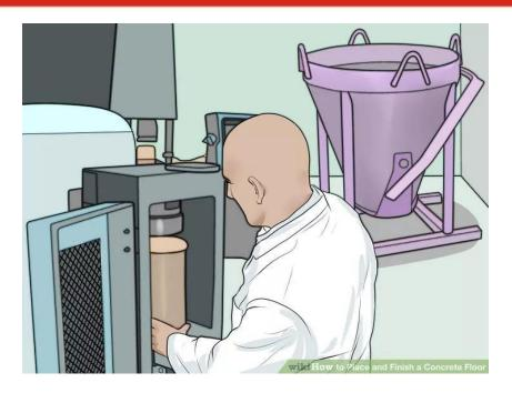
Coordinate concrete testing with a qualified testing laboratory if the construction contract requires it. Testing labs often perform the following tests:Slump. This test determines the plasticity of the concrete material. A vertical cone shaped mold is filled with concrete and the amount the concrete *slumps* is measured, to make sure it is not too wet to meet specification for the job.
