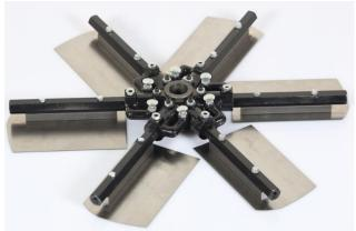
Run the troweling machines over the concrete until the level of finish you desire is achieved. For a *hard troweled* finish, you will raise the blades up on the machine as the concrete gets progressively harder, which in turn puts more pressure on a smaller area of the blade.
