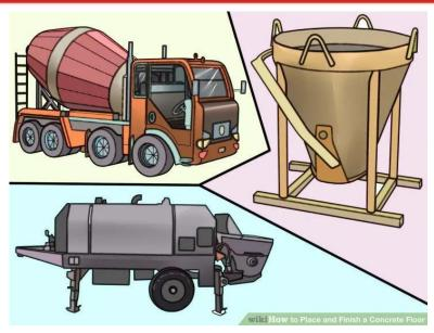
**Determine the method you will use to place the concrete in your forms.** This should be done early in the process so that concrete trucks and other required equipment will be able to get into the area they will need access to during the concrete placement. Aerial pumps can place concrete to specific areas of the slab via an articulated boom and hose assembly up to 120 feet (36.6 m) from the concrete truck. They are often used for placing concrete on elevated decks or in inaccessible locations.
