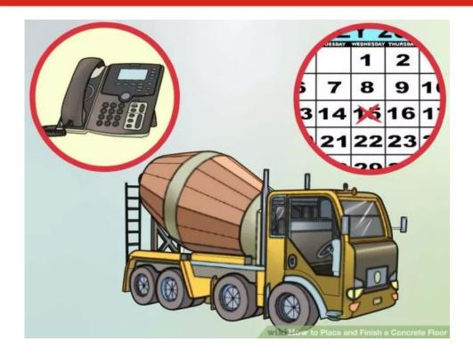
Order the concrete from a ready mix concrete supplier, and schedule the delivery to coincide with the concrete placement schedule. This means both the date and time of the pour, and the interval of delivery for multiple trucks to arrive on the job site so the concrete crew has time to discharge and tend to each truckload, while not having to wait for the next truck to arrive.
