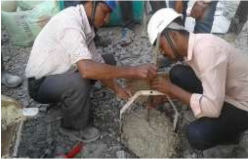
Img5 220mm slump without segregation
