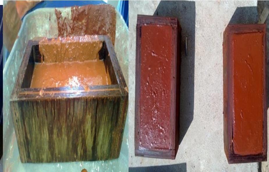
Placing of fresh composite
