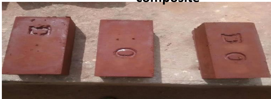
Bricks kept for curing
