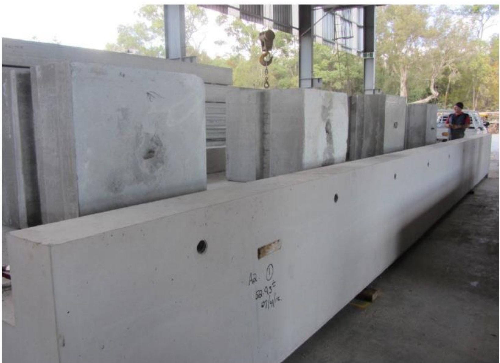
Figure 5a: Load testing of a 10 metre precast geopolymer beam.
