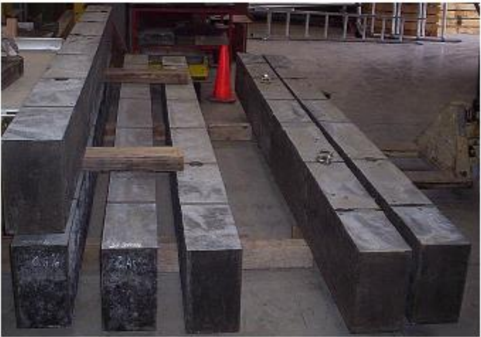
Beams after Demoulding
