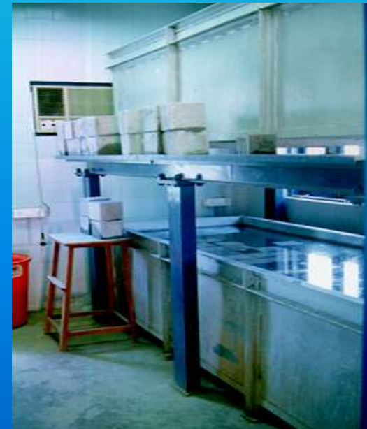
Controlled curing at 27 \pm 2^\circ\text{C}
