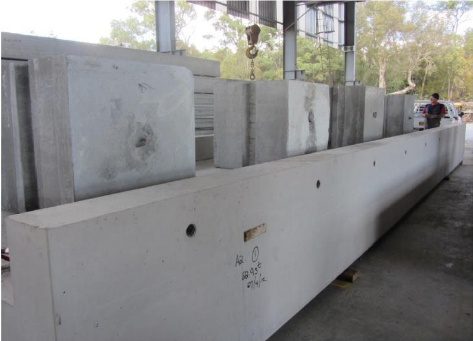
i: Load testing of a 10 metre precast geopolymer beam.
