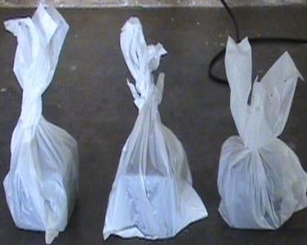
Demoulded Cubes Ready For Curing
