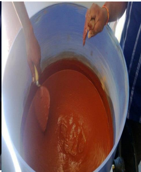
Wet mixing of geopolymer composite
