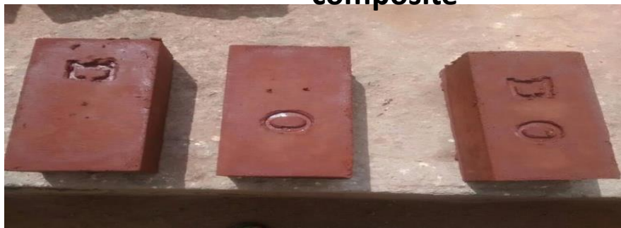
Bricks kept for curing
