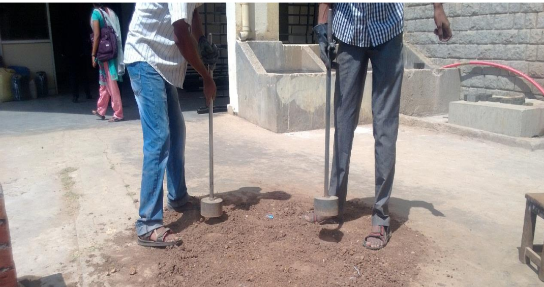
TBS BEING DRIED AND LUMPS BEING CRUSHED TBS SIEVED THROUGH 2.36MM SIEVE AND STORED
