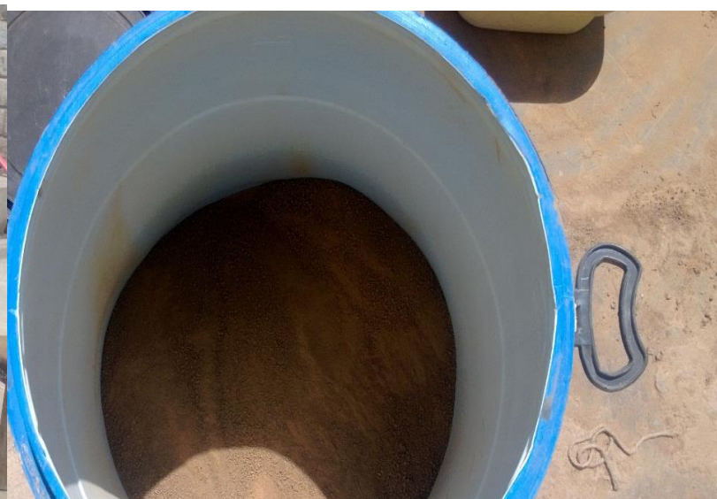
TBS BEING DRIED AND LUMPS BEING CRUSHED TBS SIEVED THROUGH 2.36MM SIEVE AND STORED
