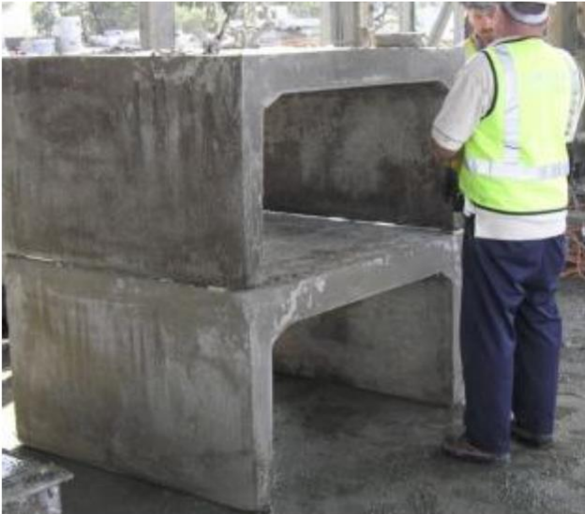
PRECAST BOX CULVERTS
