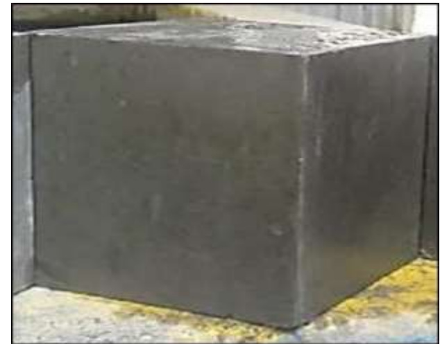
Fig. 10 : Concrete Cube with straight edges and no air voids
