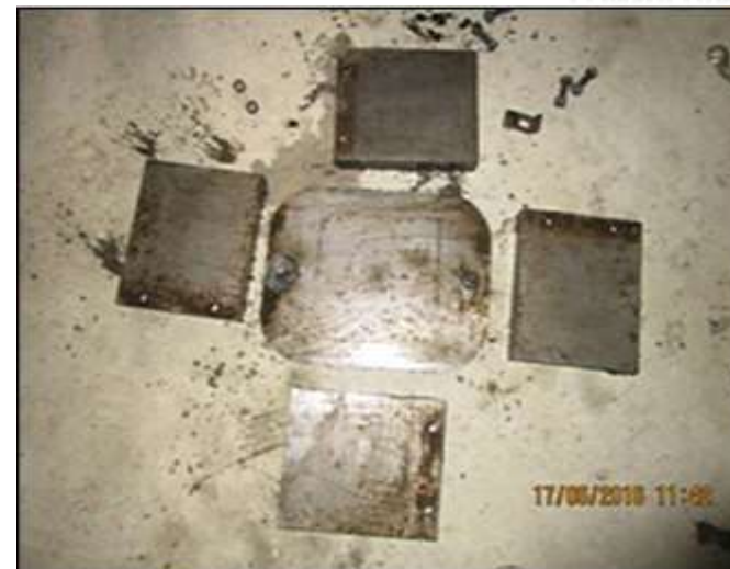
Fig. 11 : Applying lubricant to mould after de-assembling
