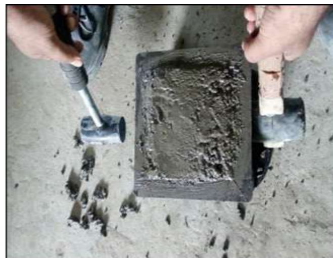
Fig. 12 : Tamping the mould by two mallets from bottom to top
