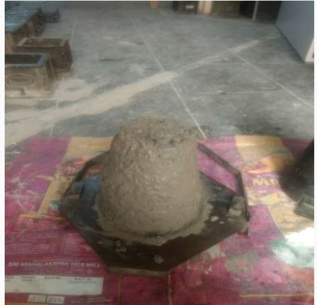
Slump cone test
