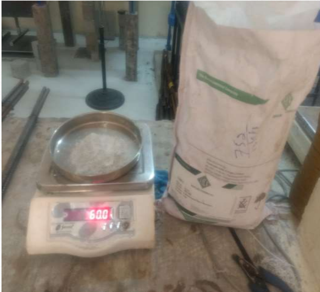
Shrinkage compensating Admixture-: EUCLID Chemical company- CONEX
