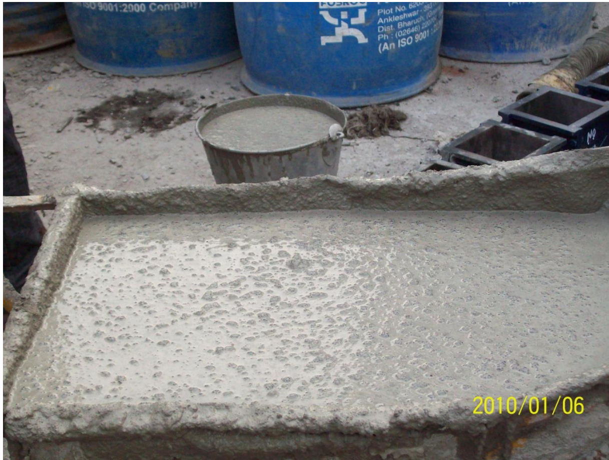
Self Compacting Concrete
