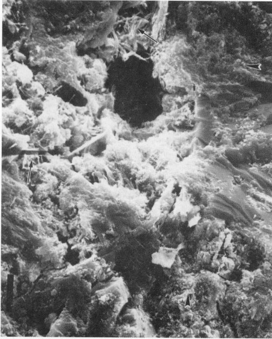
Left: An electron microscope reveals tiny flaws in a conventional mixture of concrete. These "holes" can trap water and thus weaken the concrete. Right: Fly ash particles (which look like bubbles) bind with other components in concrete to create a stronger, more durable concrete. The photographs were taken by Dr. Marcelle Gillott of UWM's Biological Sciences department.
