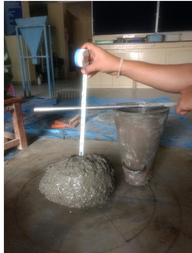
Slump of CSP-3
