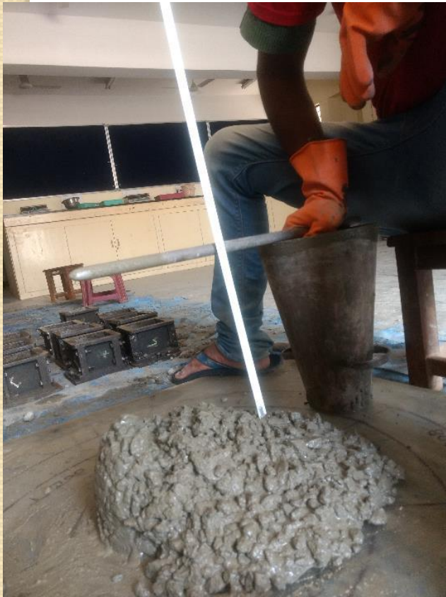
Slump of C-4/ Control-I
