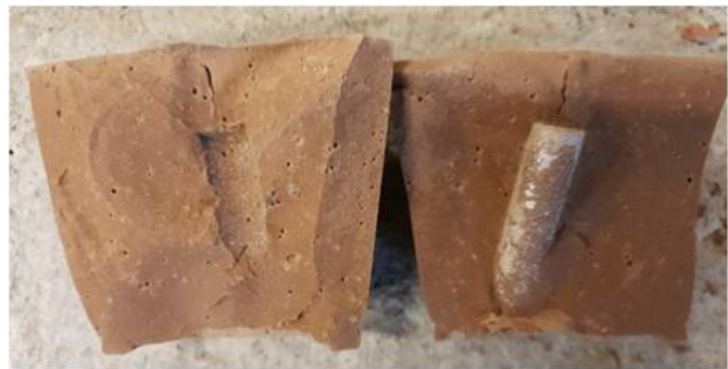
Fig. 3 - Al/5% Mg alloy rods placed in OPC paste (left) and totally converted to gibbsite after 28 days curing in moist condition, while same rod placed in paste where OPC is replaced with 55% calcined marl is in pristine condition without any corrosion products in its imprint (right).
