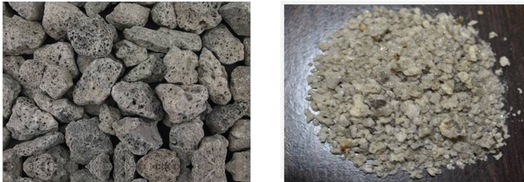
Fig 1: Air Cooled Coarse and Fine aggregates from iron slags
