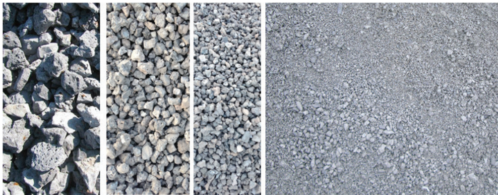
Fig 3: Air Cooled Coarse and Fine aggregates from steel slags
