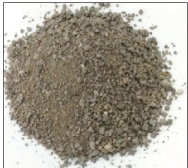
Fig 4: Steelmaking slag sand
