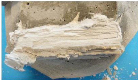
Fig. 3 - Al/5% Mg alloy rods placed in OPC paste (left) and totally converted to gibbsite after 28 days curing in moist condition, while same rod placed in paste where OPC is replaced with 55% calcined marl is in pristine condition without any corrosion products in its imprint (right).
