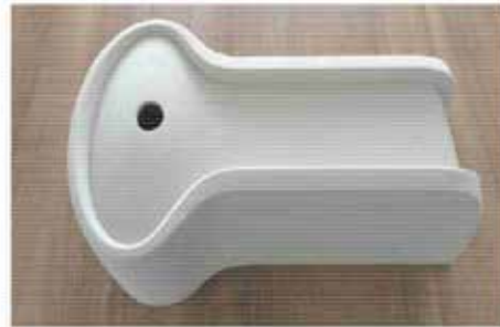
Figure 6: 3D printed concrete housing element for a prototype for Plug Charge
