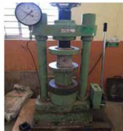
Fig. 3: Compressive loading of specimens.
