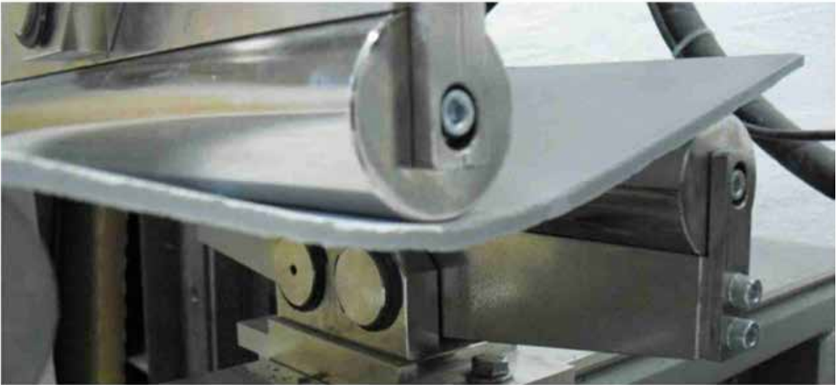
Figure 4: UPHC panel with a glas-fiber mesh, flexural strength: 73 MPa
