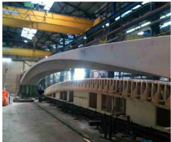
Figure 1: Goosebridge, fiber-reinforced UHPC, no steel bar reinforcement in section: Romein Beton, NL; material development: G.tecz Engineering, Ger
