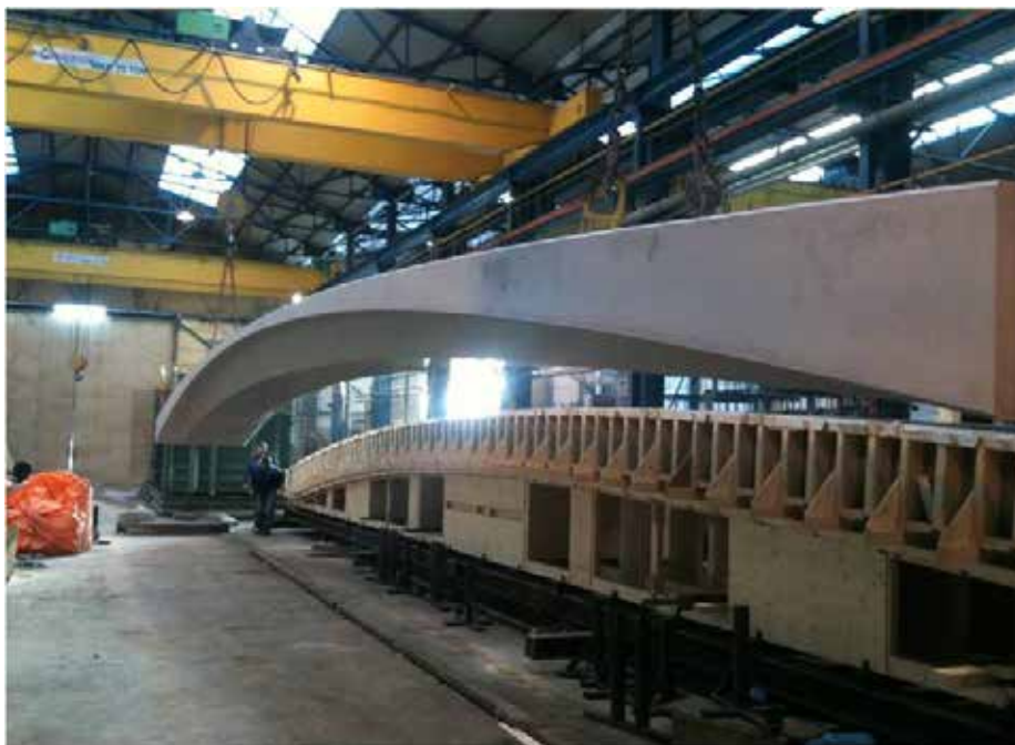
figure 1: Goosebridge, fibre-reinforced UHPC, no steelbar re-inforcement inside; production: Romein Beton, NL; material development: G.tecz Engineering, Germany
