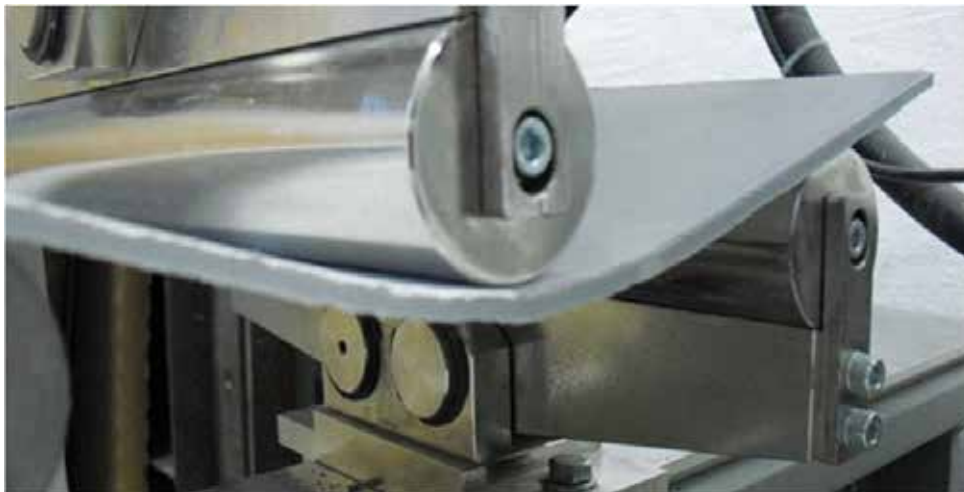
figure 4: Quantz-Pro panel with a glas-fiber mesh, flexural strength: 73 N/mm 2
