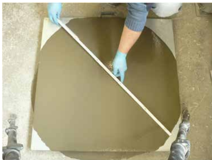
figure 5: C170 with 0.99 vol.-% steel fibers
