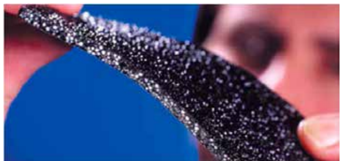
Figure 12: Non-Resin Based Bituminous Waterproof Coating
